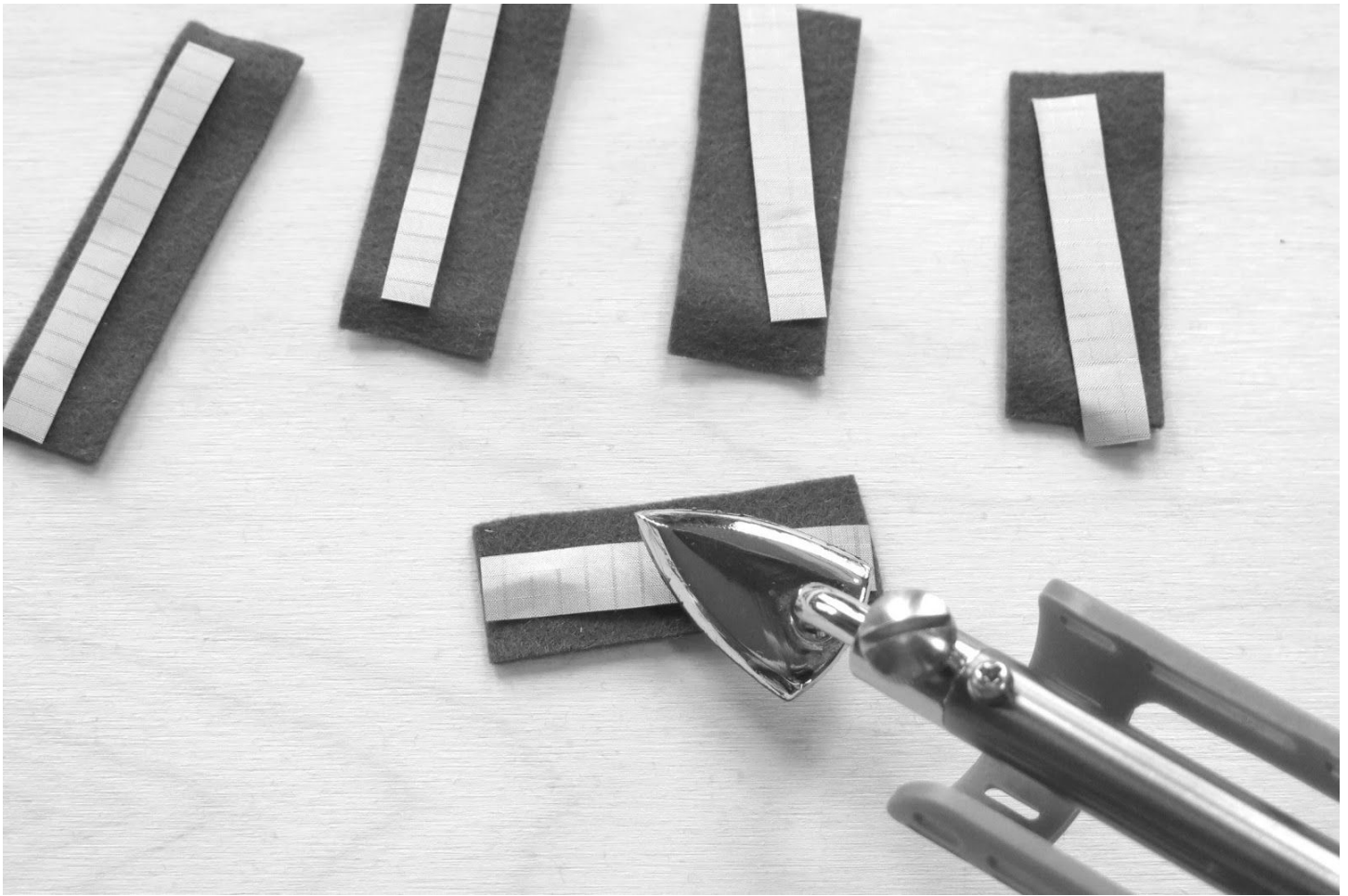
Figure 2.4 - Ironing down the conductive fabric onto the felt
