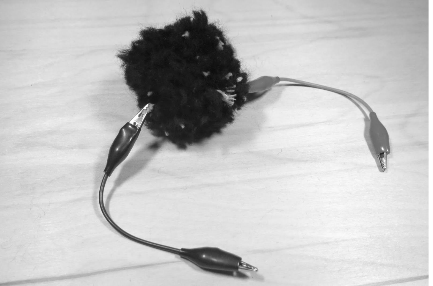
Figure 1.8 - Alligator leads clipped to conductive yarn in the pom-pom
