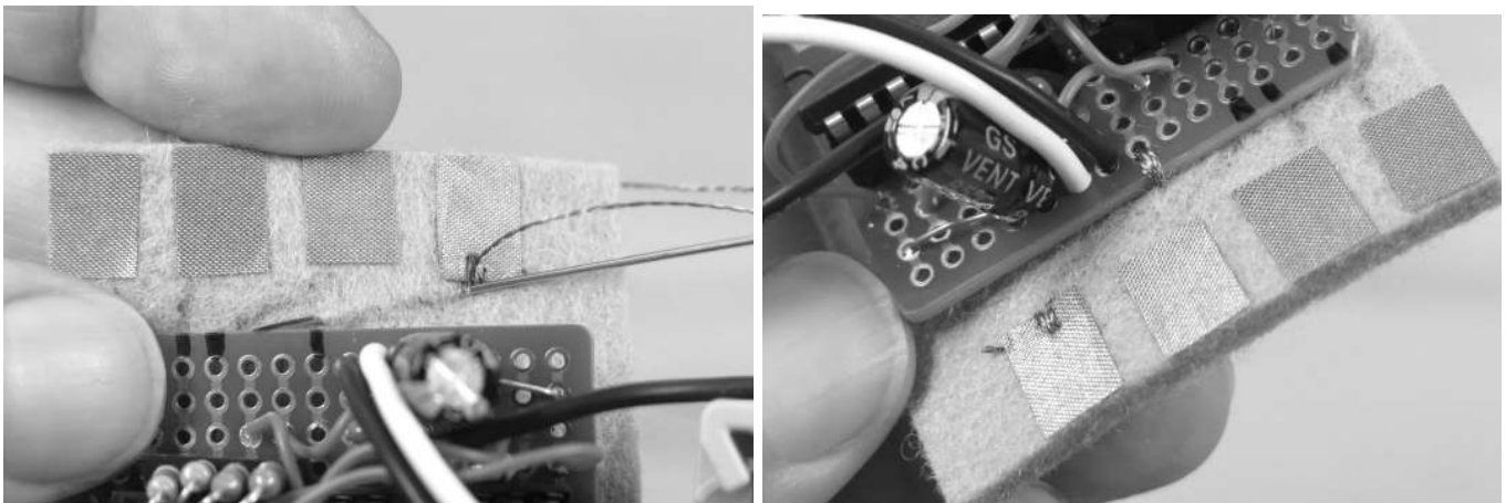
Figure 2.28a - Conductive thread stitches on conductive fabric pad, 2.28b - Conductive thread stitches going through protoboard hole
