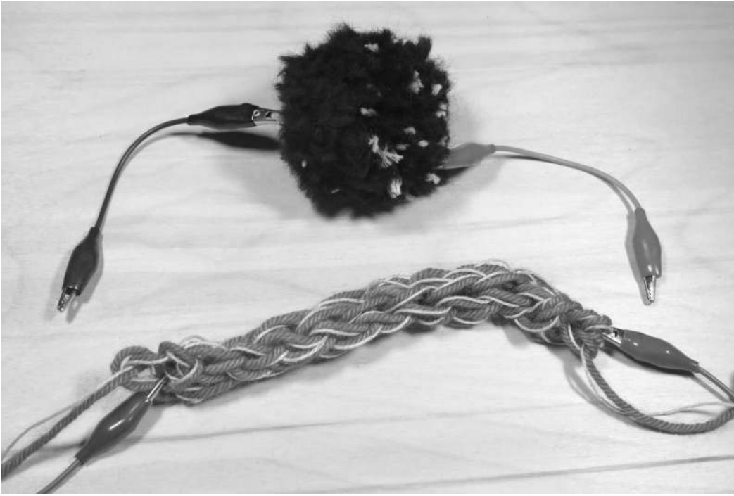
Figure 1.14 - Completed pom pom squeeze sensor and knitted stretch sensor
